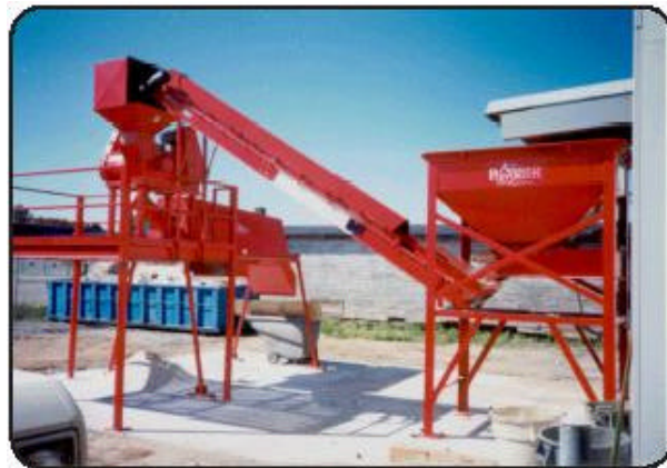
Figure 2: The Andela Glass Pulveriser with trommel and surge hopper.
