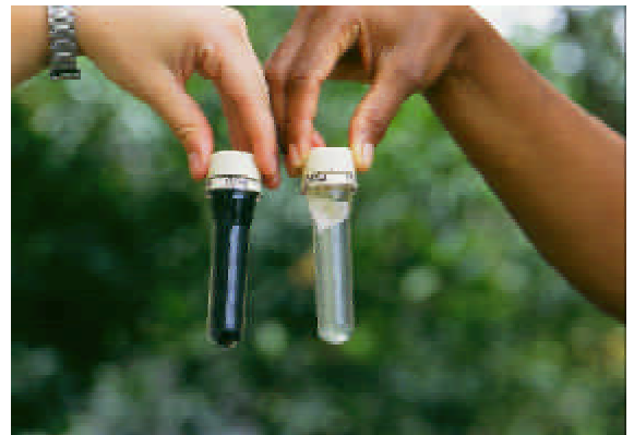
Simple presence/absence vials are being used by the Fijian communities of Vanisinu and Nalase to test their drinking water quality. This simple hydrogen sulphide strip is used to help households test their own water supplies. Water contaminated with faecal coliform turns black within a couple of days.
