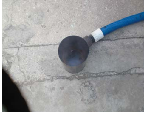
Fig 18: Flame from the gasifier – note the blue flame similar to LPG
