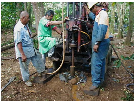
Photo- 6: Site Investigation (Exploratory Boring and Topography Survey)
