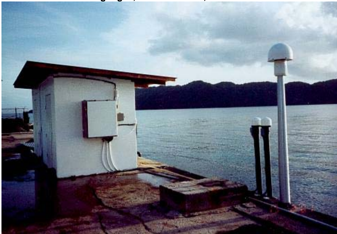
University of Hawaii tide gauge at Palau showing twin Aquatrak acoustic gauges, CGPS receiver, and instrument hut.
