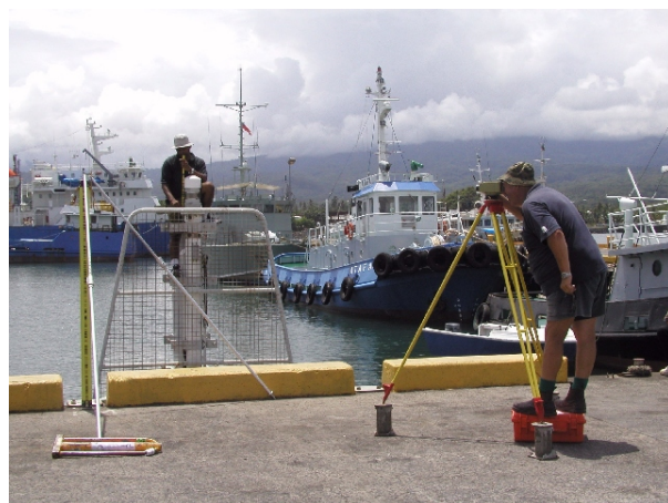
Levelling of SEAFRAME Sensor benchmark. Photo credit: Steve Turner, NTC.
