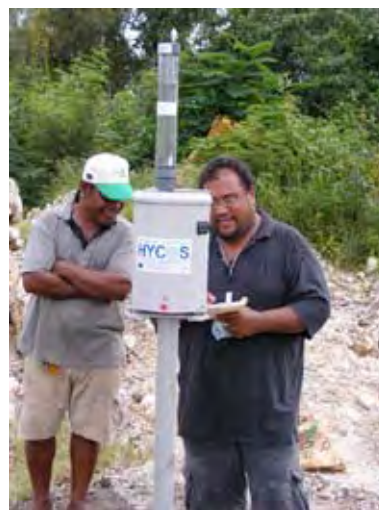
Photograph 6. calibration by ARMS personnel of the recently installed TB3 automatic rain gauge. NRC Workshop Topside
