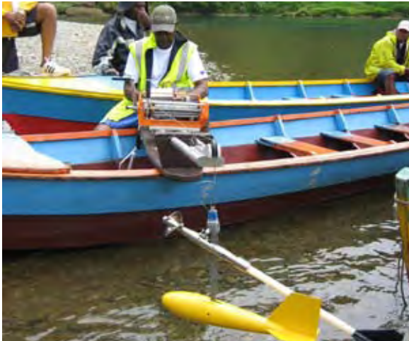
Photograph 1: river gauging equipment for flood measuring being used at Sabata Navua River
