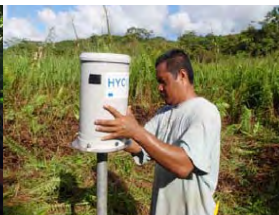
Photograph 8: installing Ngermaskang rainfall gauge
