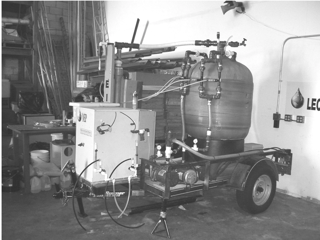
Figure 1: Photograph of the Electro-Ionization Treatment system showing the contact tank and the Clorinoxyl™ module comprising two components, the Clorin™ gas generator and the NI-OX/L™ gas generator.
