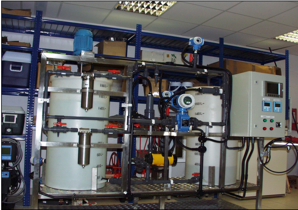
Figure 7. Lab-scale test rig for filtration performance evaluation.
