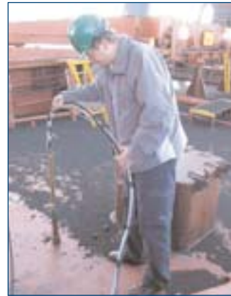
Shipboard sampling with the air-driven well pump
