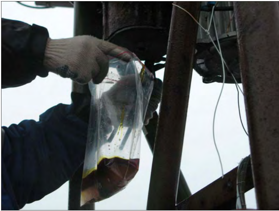
Fig. 5.5-1. Taking a sample of an utility fluid from the transformer of the locator on Site 9 (locator station), Alexandra Island
