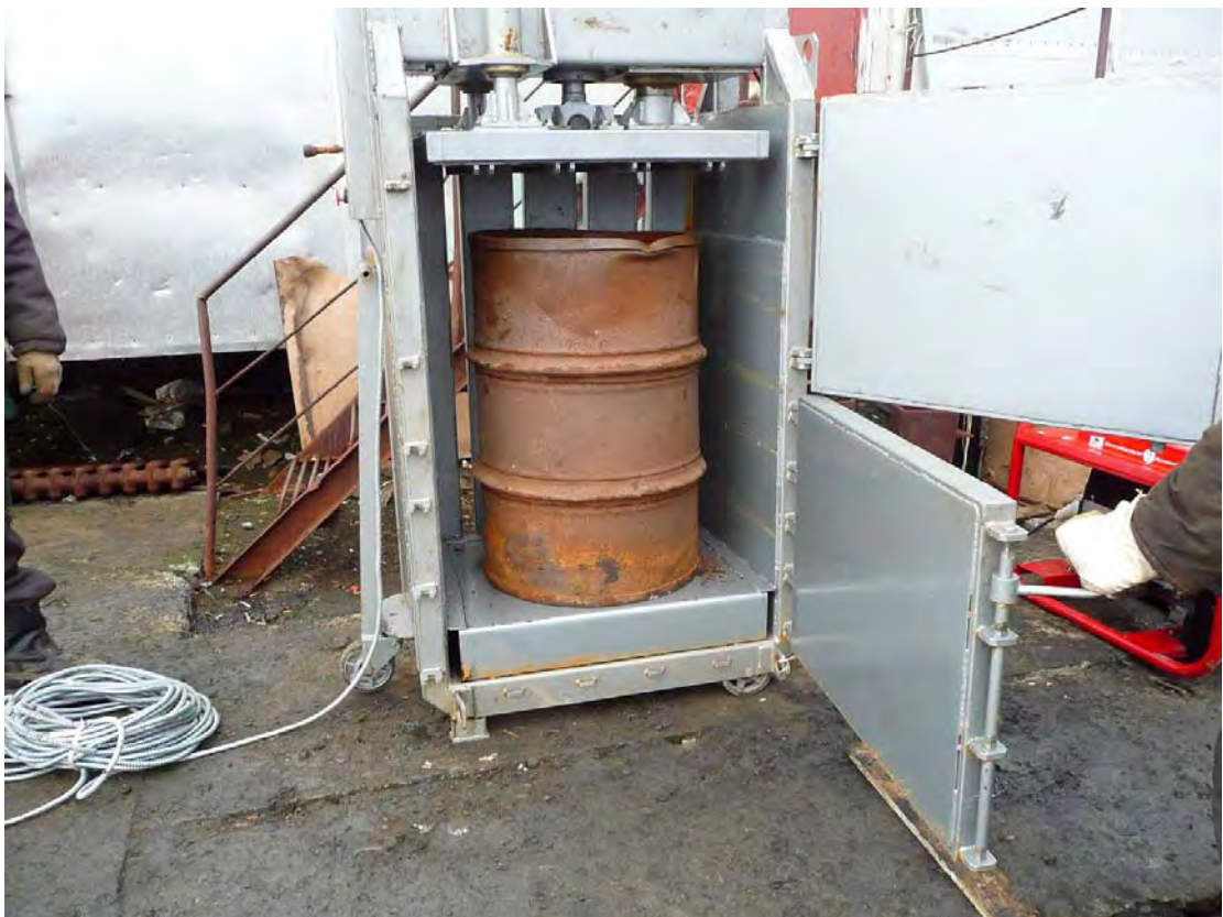
Fig. 6.3.7. The drum has had no visual changes after using the press (the dent on the top was there before the press was used on it)
