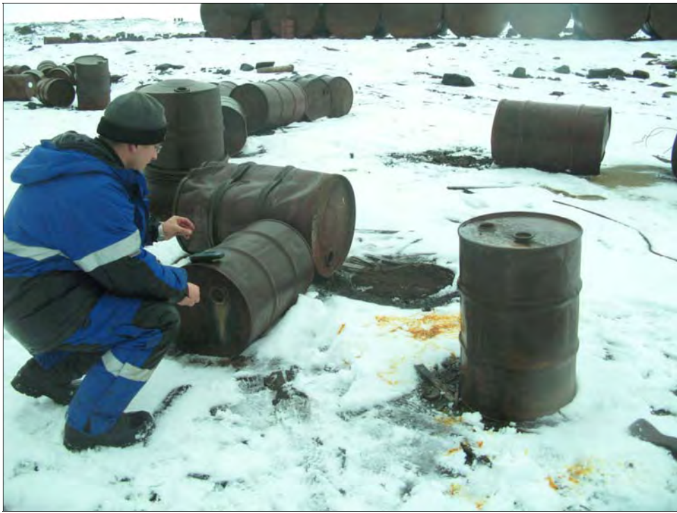
Fig. 5.5-4 Sampling utility fluids on Site 1 (Severnaya Bay fuels-lubes storage), Alexandra Island
