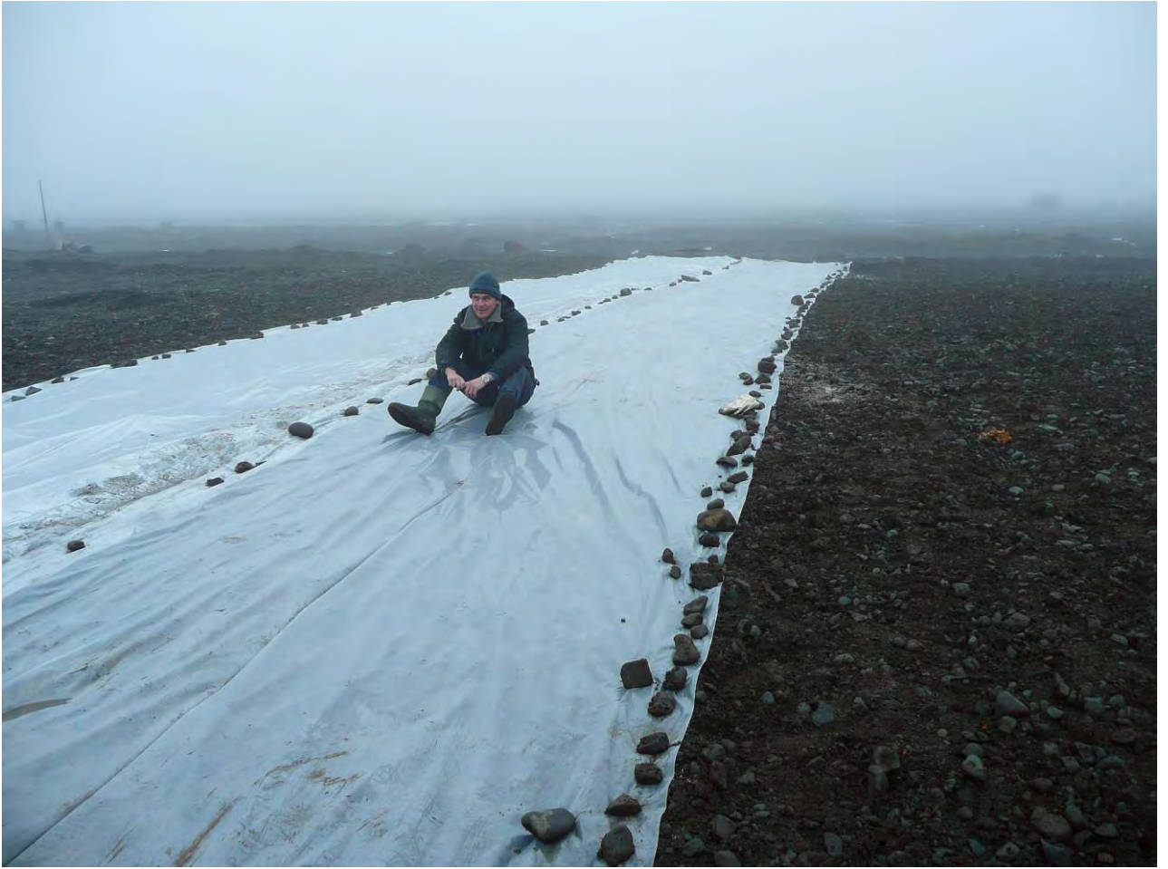
Fig. 6.3.11. A section on Pilot Ground 2 treated by biological product 'Devouroil' and covered by breathing polyethylene.
