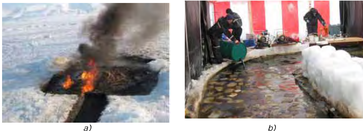
Fig.1.5. Field and laboratory experiments to study oil behavior under ice conditions and test OSR technologies: a – testing of oil burning technology at SINTEF field station (Svea Field station), Svalbard Archipelago; b – study of oil behavior under ice conditions at the Ice Laboratory (SINTEF Sealab)
