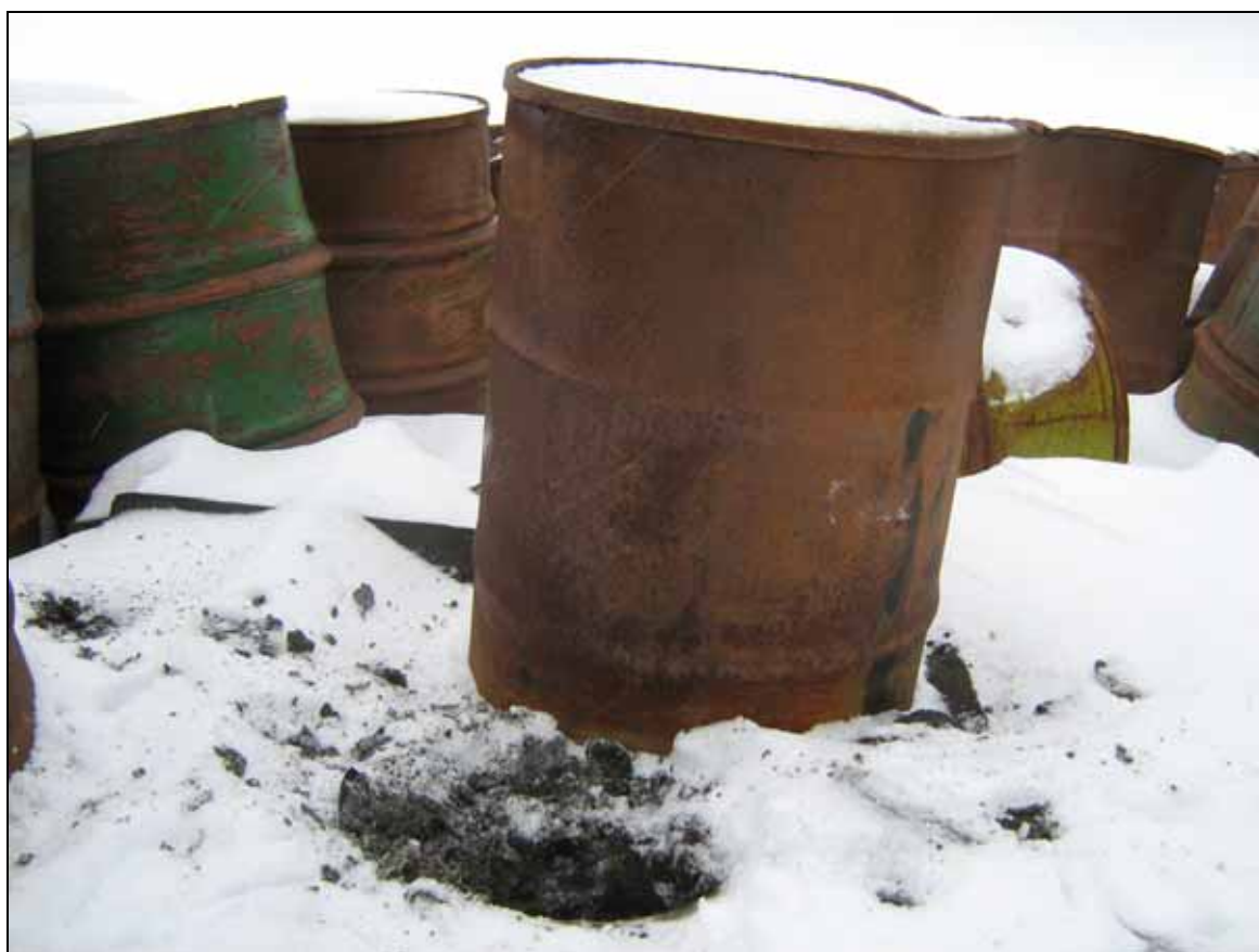
Photo 5.7 Leak of fuel and lubricants north of the empty drum storage area
