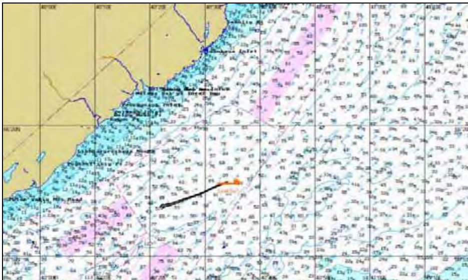
Figure 353. H+03:00. Oil slick spreading as per the scenario GC-Aut-S-2.
