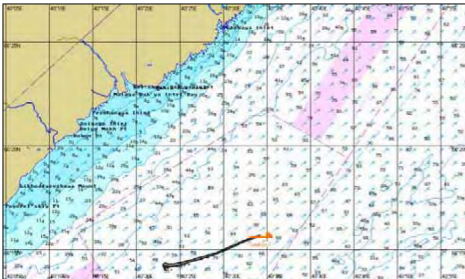
Figure 314. H+03:00. Oil slick spreading as per the scenario COU-Aut-S-2.
