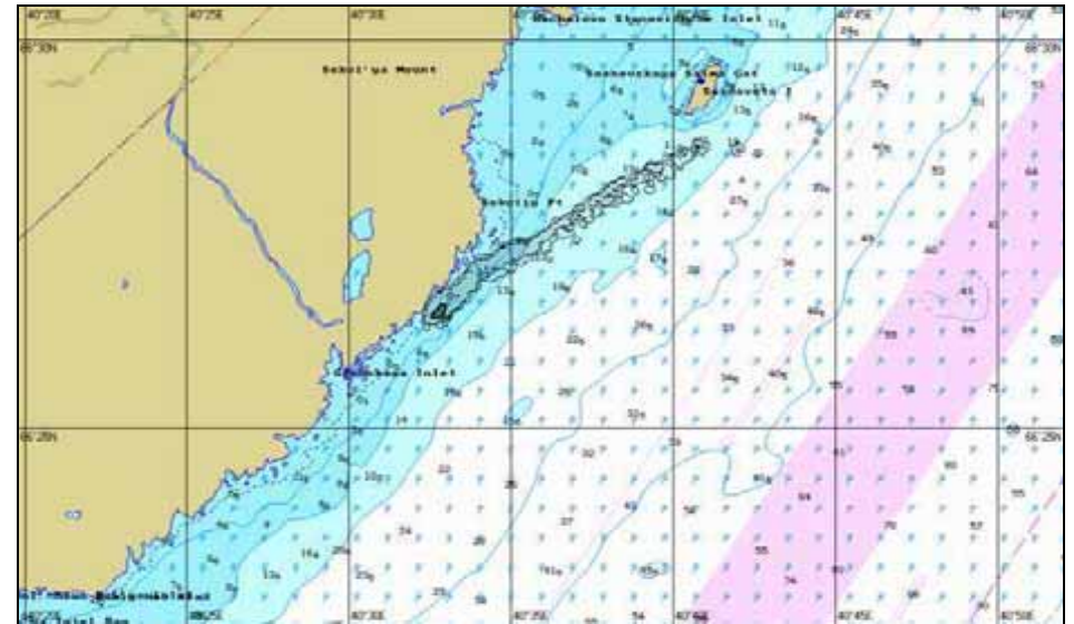
Figure 381. H+12:21 . Oil slick spreading as per the scenario Na-Aut-S-2.
