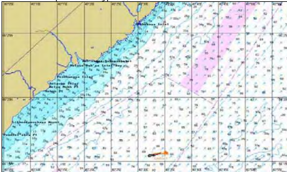
Figure 312. H+01:00. Oil slick spreading as per the scenario COU-Aut-S-2.
