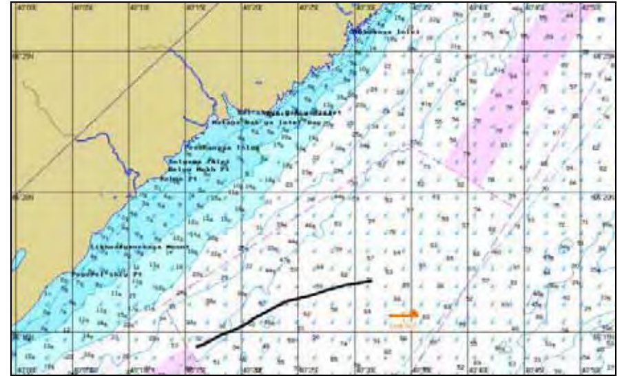
Figure 337. H+06:00. Oil slick spreading as per the scenario BO-Aut-S-2.
