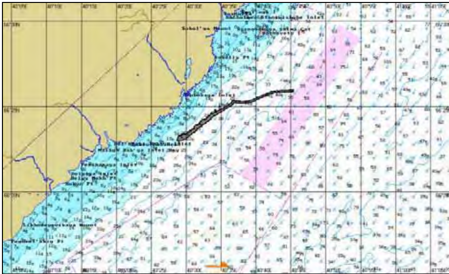
Figure 359. H+10:00. Oil slick spreading as per the scenario GC-Aut-S-2.
