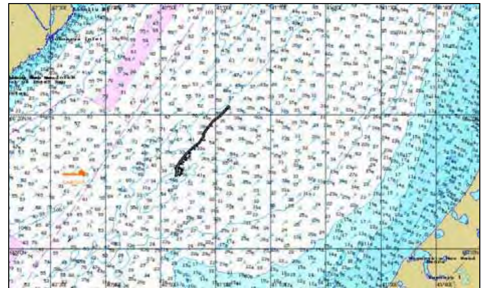
Figure 400. H+15:00. Oil slick spreading as per the scenario COU-Aut-W-2.
