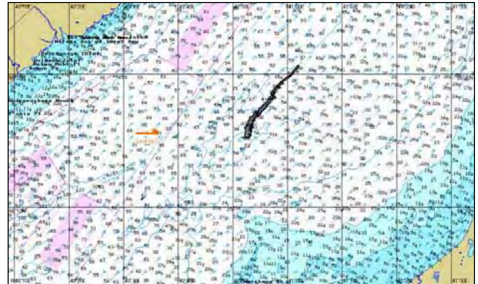
Figure 436. H+15:00. Oil slick spreading as per the scenario GC-Aut-W-2.
