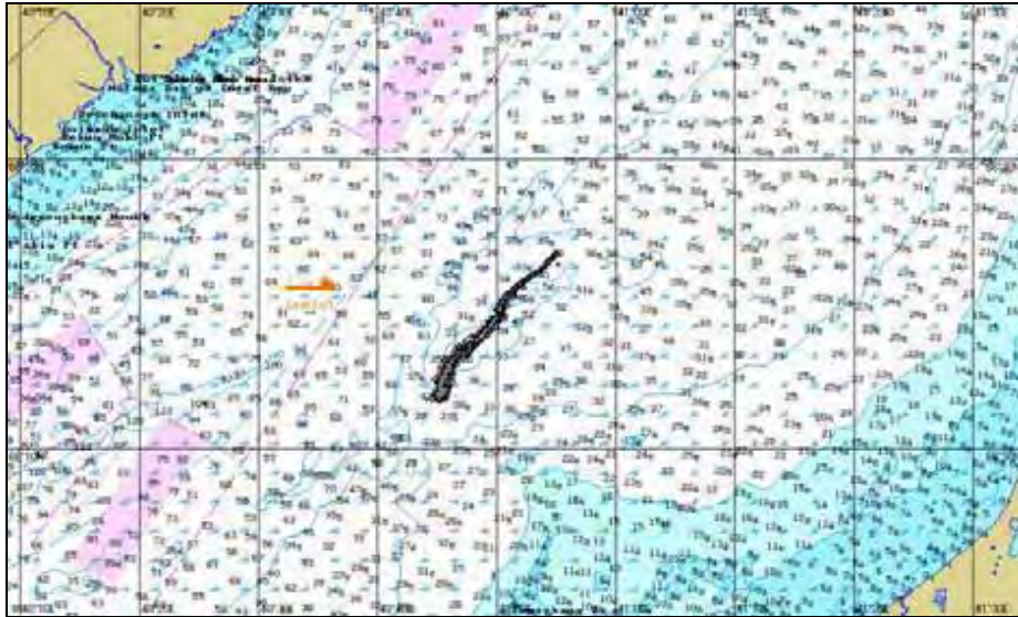
Figure 437. H+18:00. Oil slick spreading as per the scenario GC-Aut-W-2.
