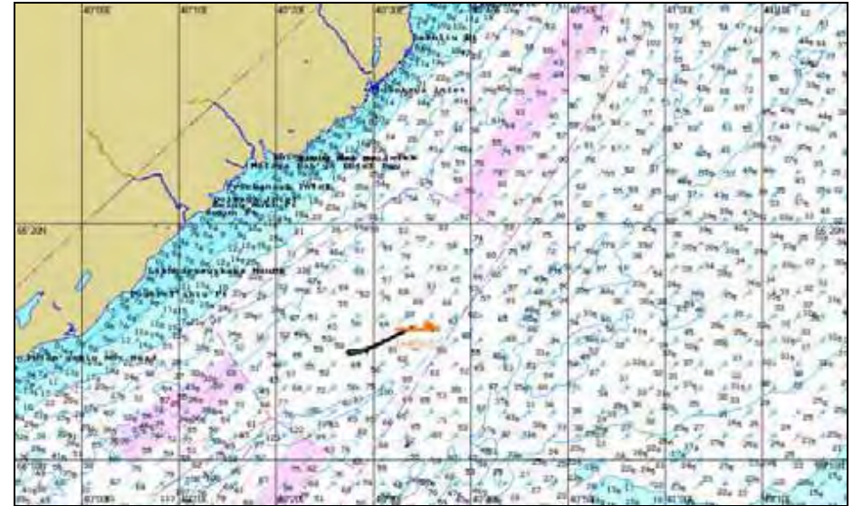
Figure 352. H+02:00. Oil slick spreading as per the scenario GC-Aut-S-2.
