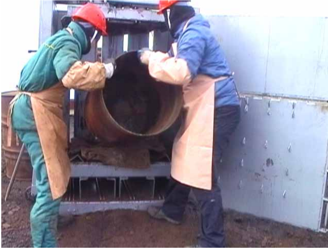
Figure 14.3 Placement of burnt drums in the press without closing gate
