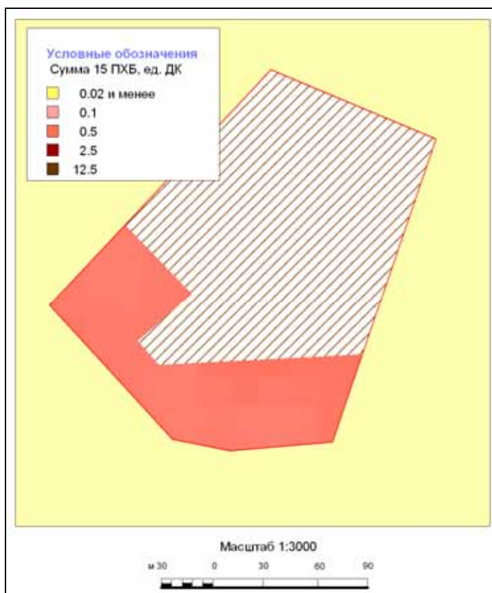
Figure 5.2.7 Spatial characteristics of the level of soil contamination of territory of the abandoned polar station PCB
