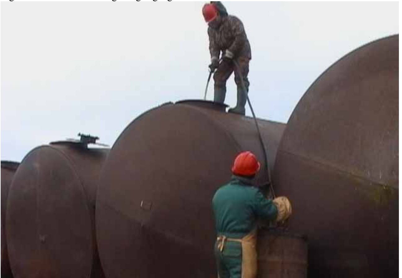
Figure14.8. Liquid transfer to a 25 t cistern
