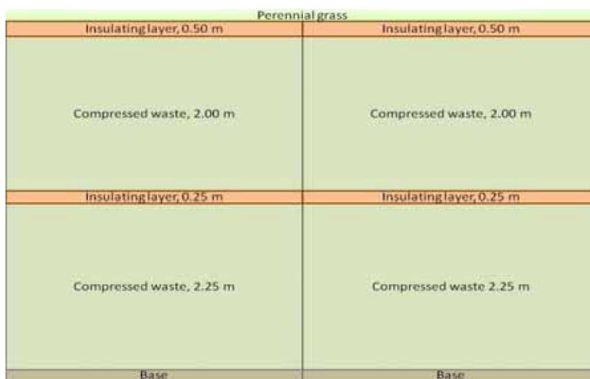
Figure 4: The construction of 2 neighbouring cells.
