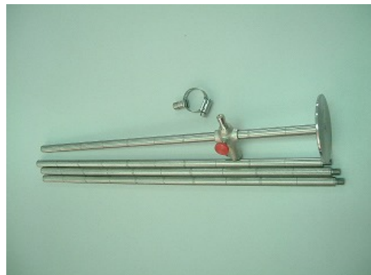
Photo 4: Flow Meter Equipments
