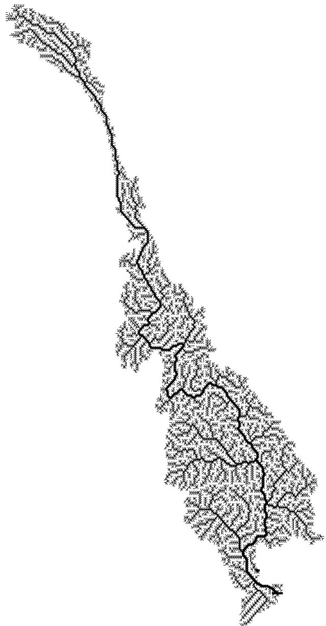
Figure 2. Mekong 1/12° (5 arc-minutes) resolution stream network, used for the routing of simulated runoff
