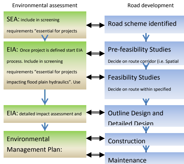
Figure 1 Relation between road development and environmental assessment steps after the Master plan stage.
