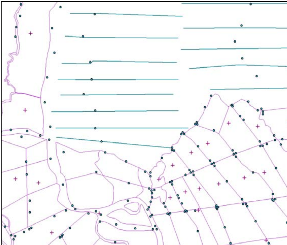
Figure 2.34 ISIS calculates with (among others) reservoir nodes (+) and cross-section nodes (dots). A spatial component of ISIS contains cross-sections (blue lines) and reservoirs (purple polygons). However, the relation between the calculation nodes and the lines/ polygons may not always be one-to-one if the GIS-files are not updated.
