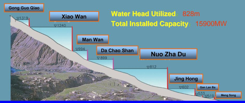
Development scheme: 8 cascades with 2 large reservoirs Tasks: Electricity generation mainly, navigation, flood control and water supply
