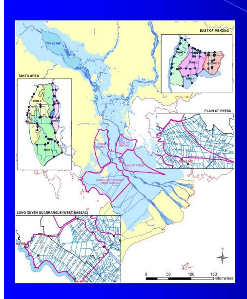
Foreseeable Future scenario, up to the year 2030, in which the existing agreed plan for flood protection in the Mekong Delta in Vietnam is expected to be completed, and a mix of early and full flood protection in the Cambodia part of the delta is considered (FMMP C2).
