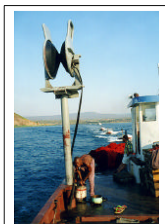
Figure 35 The hydraulic power block on a purse seine boat based in Mpulungu
