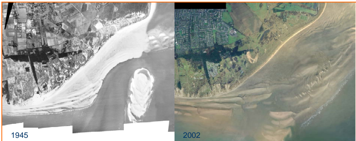
Figure 5. Human alteration of coastal processes. Dredging of the River Mersey, UK and the construction of training walls have altered sediment movement leading to erosion/accretion zones and closure of a channel in the area south west of Formby known as Taylors spit and the Formby channel between 1945 and 2002.
