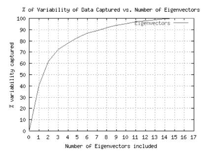
This example shows a typical eigenvalue plot. Depending upon your point of view, it would be possible to argue that anywhere from 4-10 of the principal components are important. The principal components from 10-17 account for less than 5% of the variability of the dataset.
