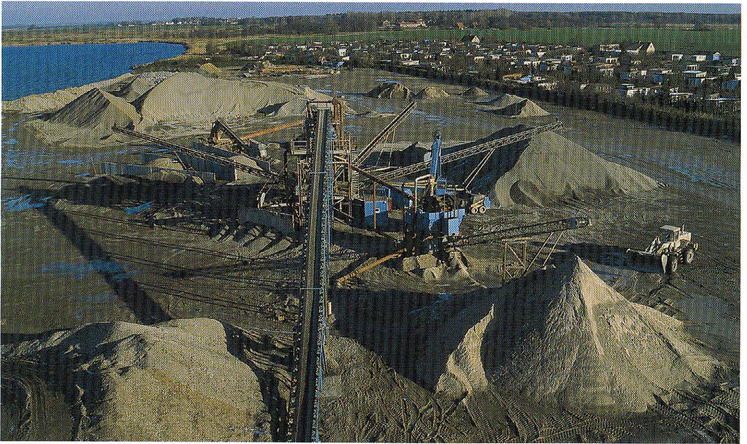
Figure 4: Use of marine sediments: Industrial raw material. Landing and processing facilities near Greifswald (Germany) (by C. Herrmann).
