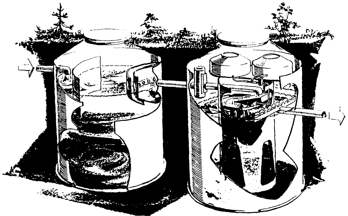
Figure 2 Mini-plant (WALLAX) for chemical treatment
