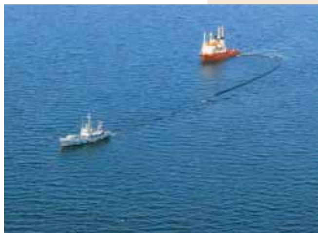
Danish "Gunnar Seidenfaden" and Estonian "Triin, PVL 200" towing a boom.
