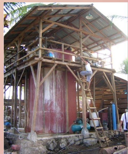
Cyanidation of amalgamation tailing.
