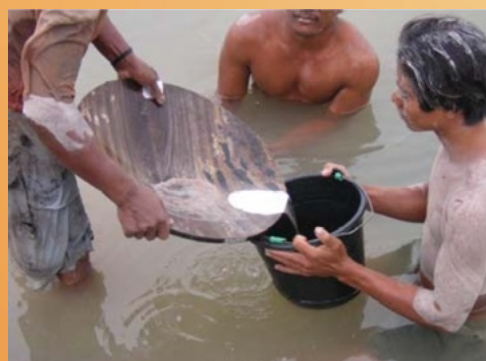
Recovering mercury after amalgamating a concentrate.
