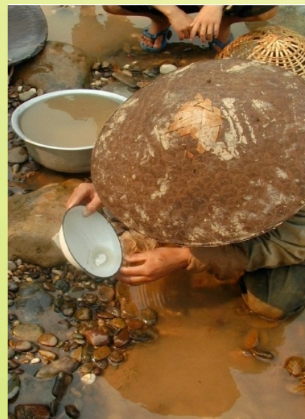
Collecting amalgam from a pan concentrate
