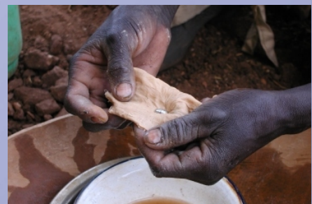
Squeezing off excess mercury.
