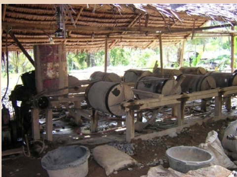
Whole ore amalgamation with trommels.
