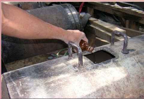
Pouring mercury into a trommel mill.
