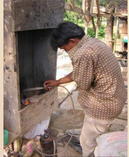
Burning amalgam without a retort.
