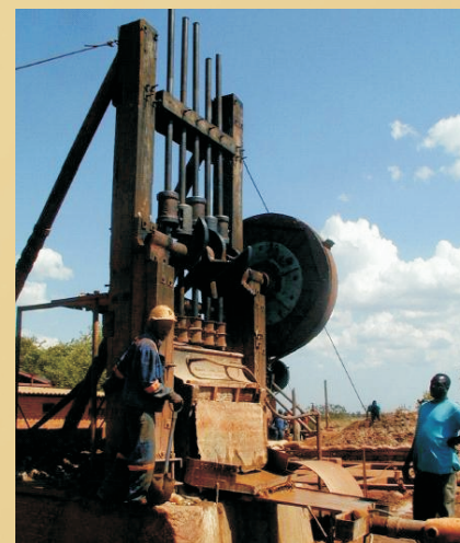
A typical stamp mill and copper plate amalgamation centre.
