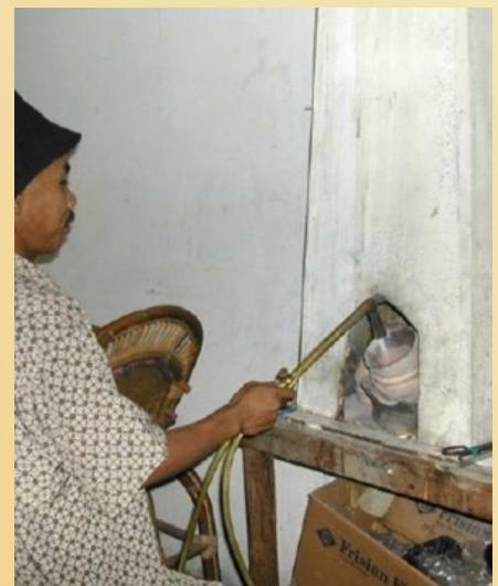
Burning amalgam without a retort.
