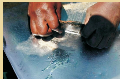
Scraping amalgam off a copper plate.
