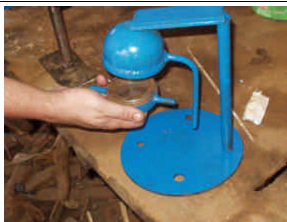
Other type of retort locally manufactured
