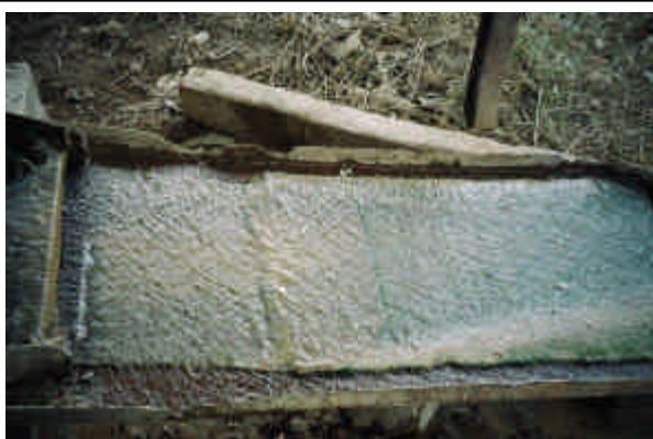
Carpets (introduced by UNIDO) replacing Cu-plate to concentrate gold
