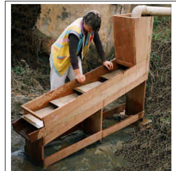
First box built to support Goldtech plates
