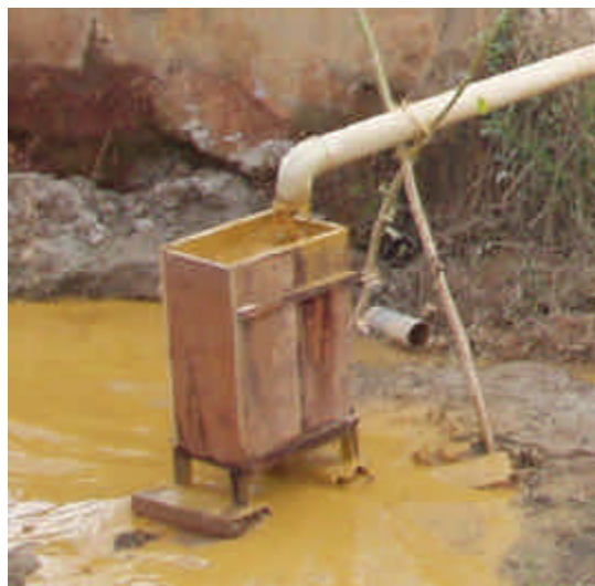
Second (zigzag) box built to support Goldtech plates
