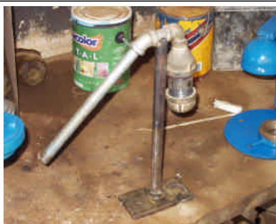
Home-made retort made of water pipes
