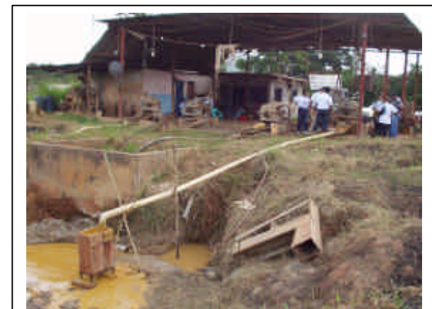
El Mago Processing Center: Goldtech plates reducing Hg emissions
