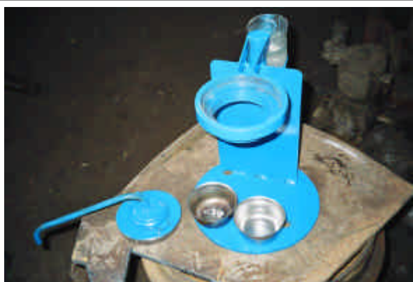
Retort locally made using kitchen stainless steel bowl
