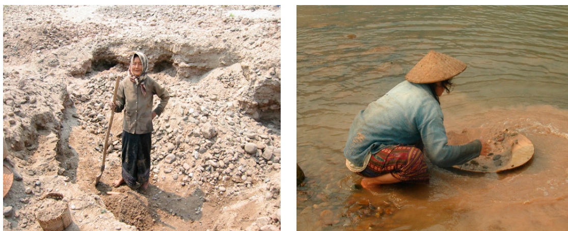
Figure 7 - (a) Houay Gno digging of the alluvium in the riverbed of the Mekong; (b) panning of the alluviums.
