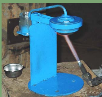
Step One: Use retort to burn the gold safely
