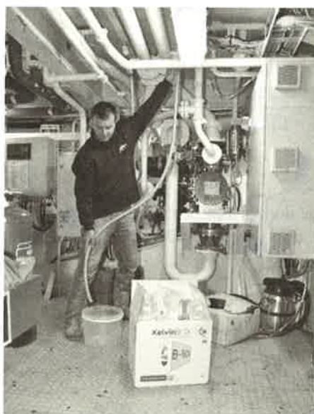
Figure 1. Sampling ballast water on board the RV Pelagia. The sample bottles are sent in the B-box to the ship by NIOZ. After sampling the bottles are sent back to NIOZ in the cooled B-box in the front. The number and contents (fixatives) of the bottles vary depending on the analyses that have been requested.
