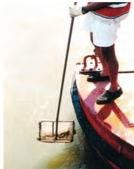
Pictures 7 and 8: Pole scraper used in India
