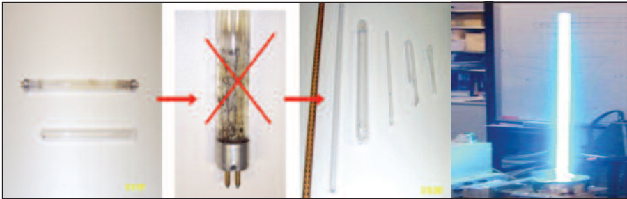
Figure 1. Microwave-powered electrode-less UV bulbs
