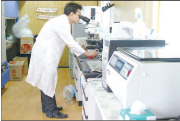
Figure 9. The barge-mounted laboratory allowing on-site biological analysis of ballast water samples following each Test Cycle.
