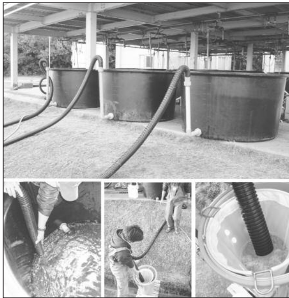
Figure 5. One m 3 -capacity tanks (upper photo) tentatively storing the treated water for L-size organisms. The water in the tanks were siphoned out and concentrated through plankton net (lower photo)
