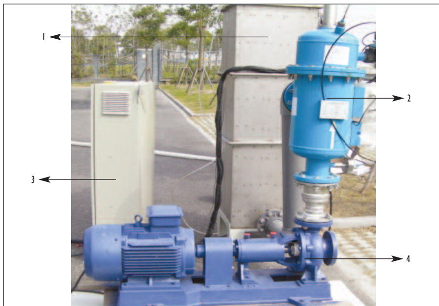
Figure 4. Picture of One Module of VUV Photolysis BWM System Prototype 1. VUV photocatalysis Reactor 2. Self-cleaning Filtration System 3. Automatic Control System 4. Assistant Pump for Onshore Testing mimic a ballast pump
