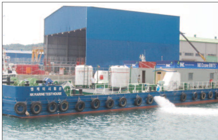
Figure 8. The mobile barge used for full-scale land-based testing of the NK-O3 system, moored alongside in Busan port. The two large white feed tanks can be seen on deck. The NK-O3 system is fitted below decks. In this picture the system is deballasting, as indicated by the ballast discharge at lower right.
