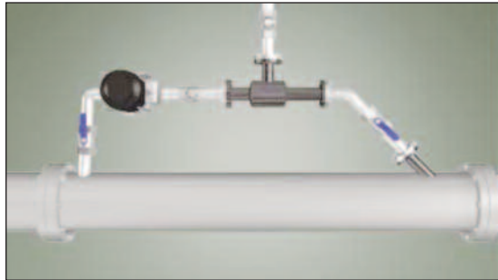
Figure 4. Ozone (side-stream) Injector (Source: NK)
