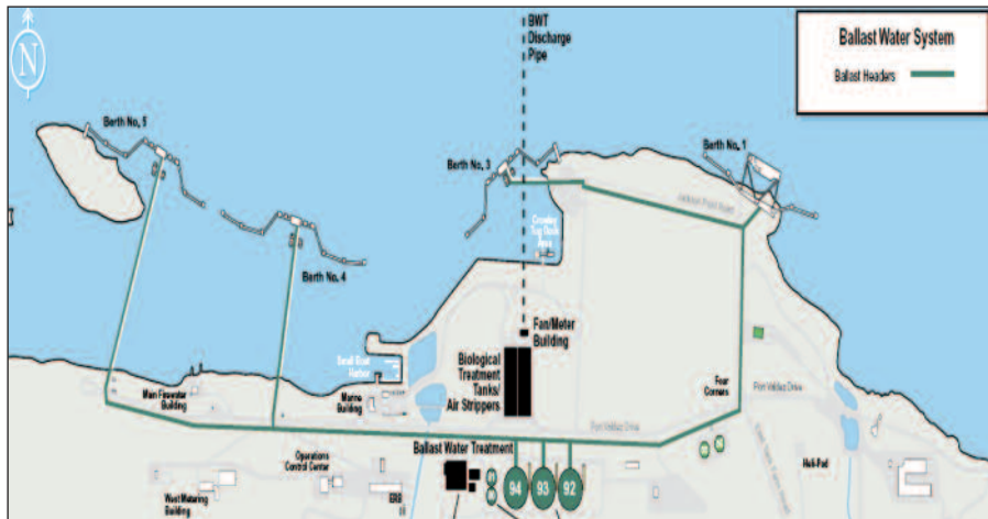
Figure 3. Ballast water system at Valdez Terminal (Source: OASIS Environmental Inc, 2004)
