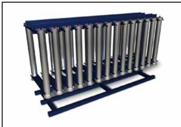
Figure 8. Ionization generator rack module for Carnival Elation current system.
