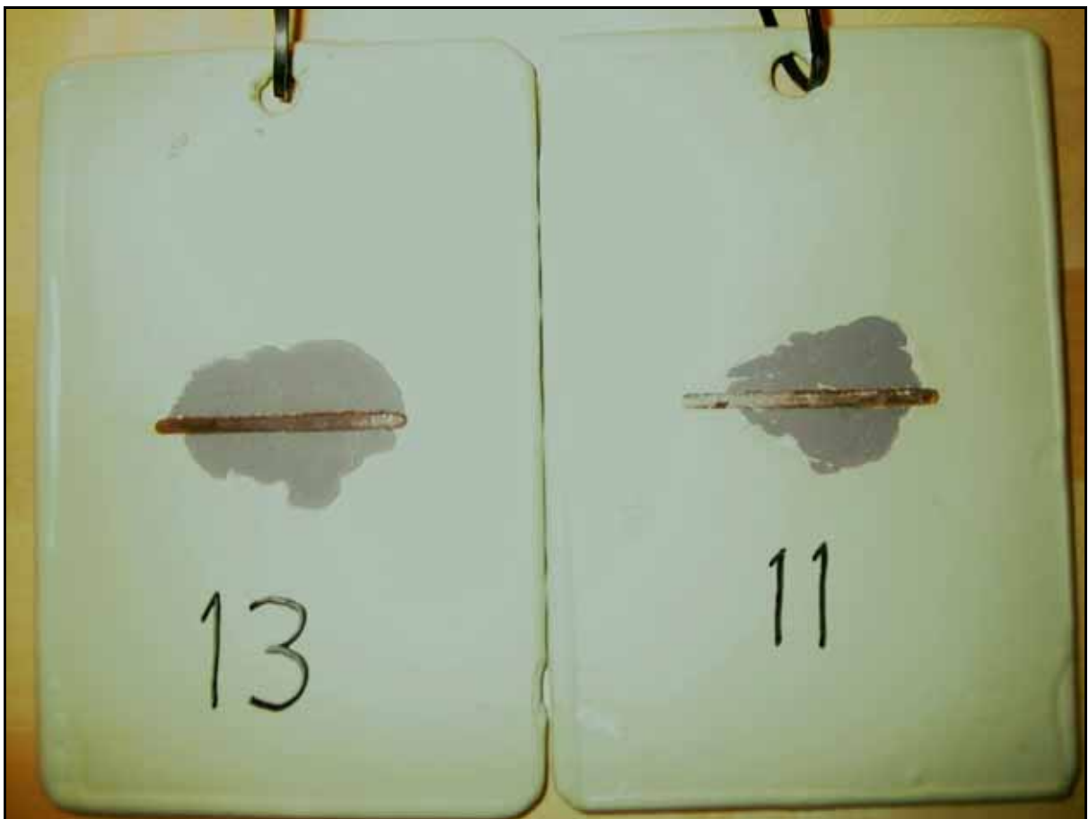
Figure 2. Coated coupons with scribed surface showing disbonding of coating after ozone treatment.
