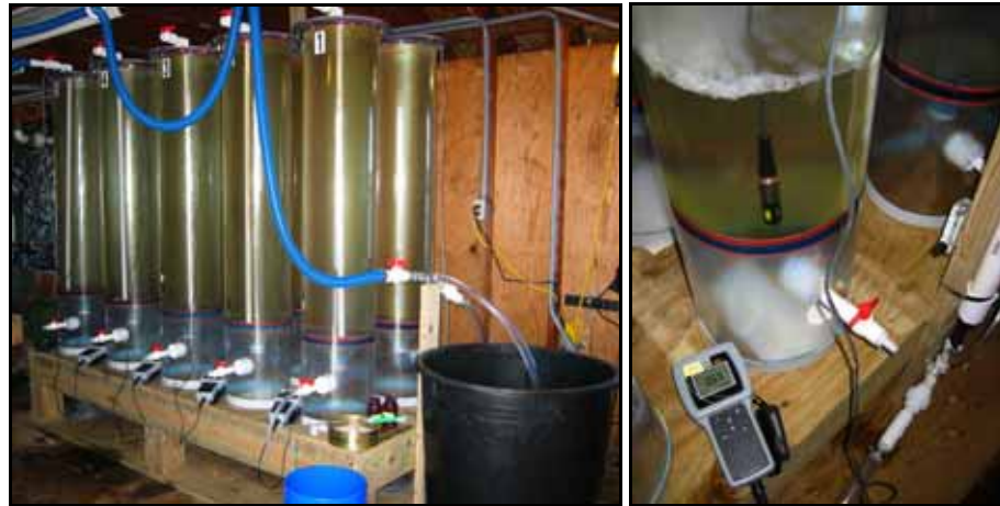
Figure 1. Mesocosm experimental setup to examine the effectiveness of Venturi Oxygen Stripping™ at killing natural planktonic organisms found in Chesapeake Bay.
