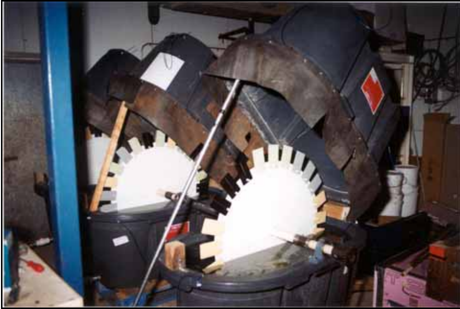
Figure 1. The test tanks set up with test coupons at the start of an experiment.
