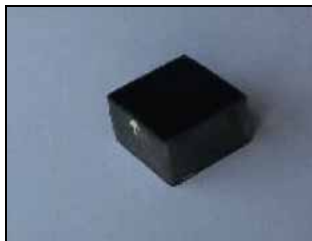
Figure 3. \text{YBa}_2\text{Cu}_3\text{O}_7 bulk superconductor impregnated with epoxy resin (20 mm thick). Eleven such bulk magnets form a 387-mm-long trial HTS bulk magnet.
