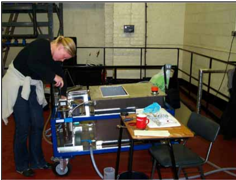
Figure 8. Laboratory Scale Advanced Oxidation Technique.
