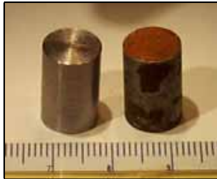
Figure 1. Electrode to the right was exposed to ozone treated water in one test compared to untreated electrode.
