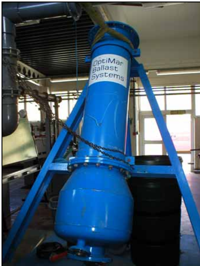
Figure 4. Ballast water equipment of Optimar during installation in the test facility at the University of Hertfordshire.
