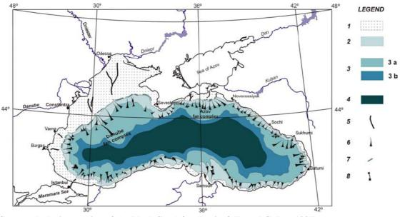
Fig. 1 – Geomorphologic zonation of the Black Sea (after Panin & E. and G. Ion, 1997) Legend; 1, continental shelf; 2, continental slope; 3, basin apron: 3 a - deep sea fan complexes; 3 b - lower apron; 4, deep sea (abyssal) plain; 5, paleo-channels on the continental shelf filled up with Holocene and recent fine grained sediments; 6, main submarine valleys - canyons; 7, paleo-cliffs near the shelf break; 8, fracture zones expressed in the bottom morphology.
