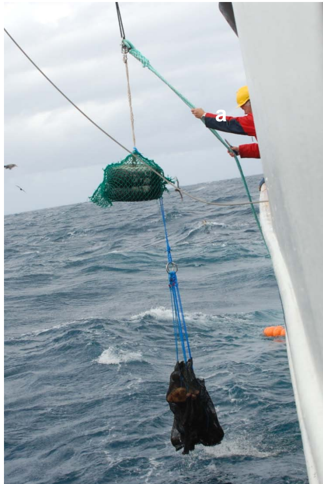
Figure 10.5 The moorings were deployed by the ship's crane over the side of the ship.
