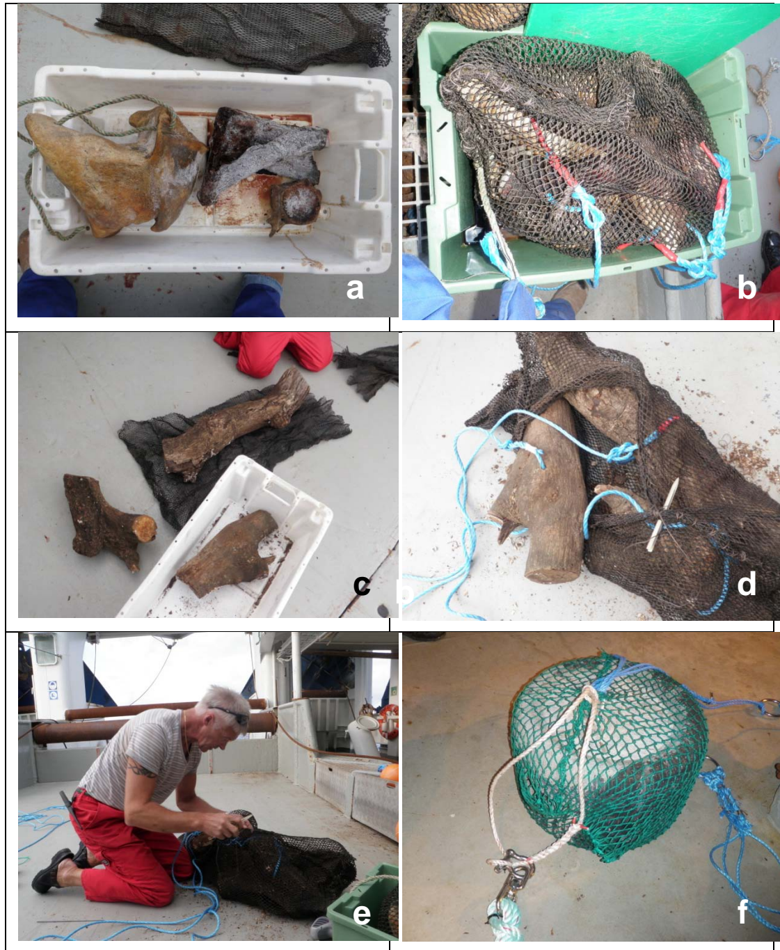
Figure 10.2 Mooring preparation. (a -b) Bones were drilled and fitted with individual loops of line. They were then sewn up into mesh bags. (c-d) Wood was prepared in the same way. (e-f) These lines were fitted to lifting rings (visible in the right of image f) which were attached directly to the ballast.
