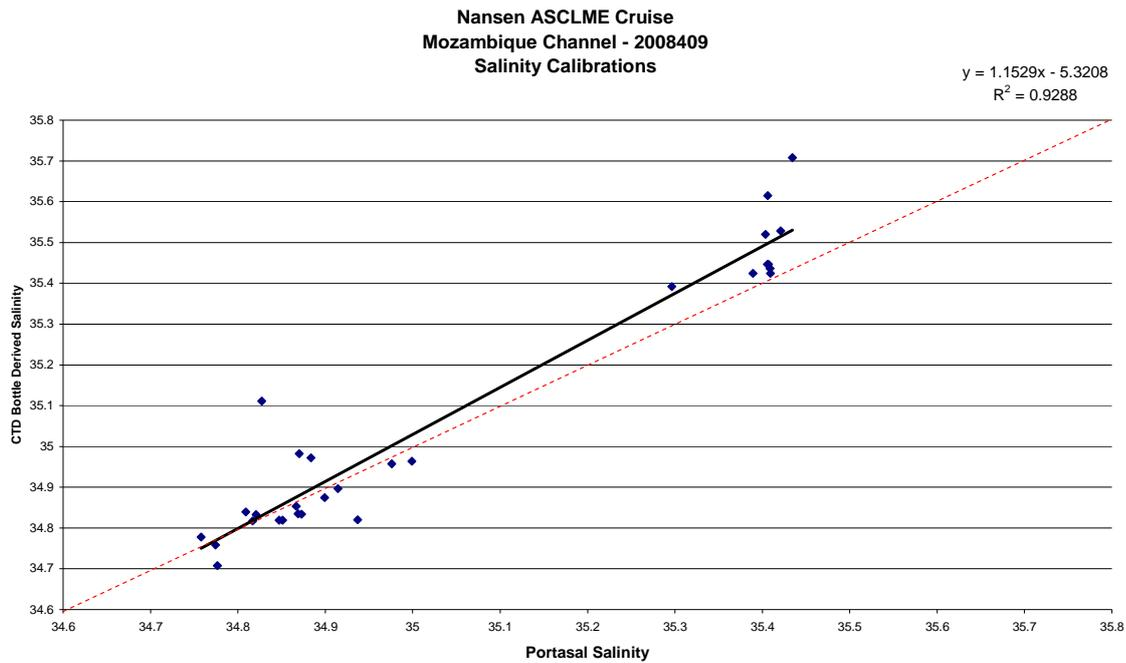
Figure 2.1.1b. Derived salinity regression plot – CTD bottle salinity vs. Portasal Salinity readings.
