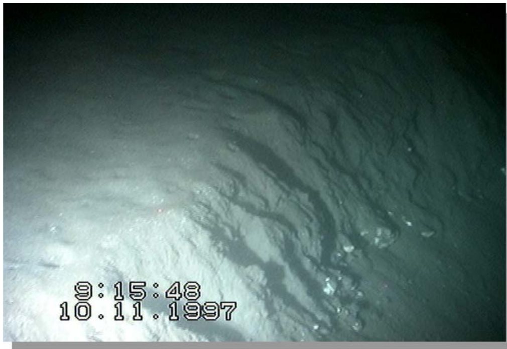
Plate 1. Seabed video image of a mined area taken using the Jago manned submersible showing the edge of a mining block with a 0.5m thick mud layer covering the 0.2m thick target gravel layer. Some subsequent slumping of the fine surface sediments into the excavation is evident.
