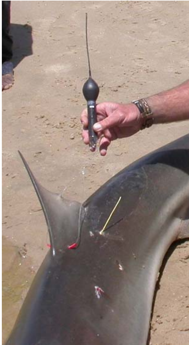
Picture 2. A Pop-up Satellite Archival Tag (PSAT) attached to the dorsal fin of a bronze whaler with a harness. Note conventional yellow dart tag too.
