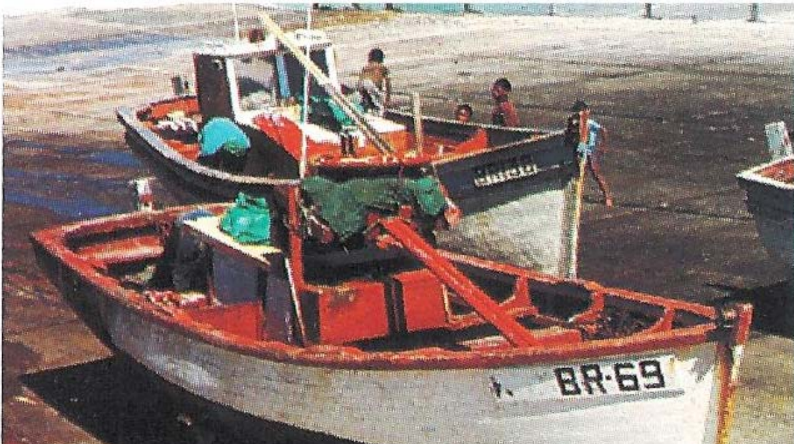
Figure 4: Example of several ‘catrongas’ with or without cabins, with inboard engines
