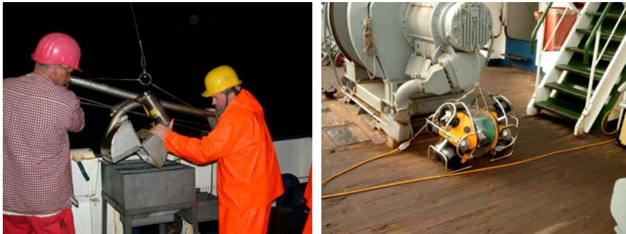
Fig. 21 : The macro-zoobenthos was sampled by a 0.1 m 2 van Veen grab (left). For imaging and assessing the underwater habitat a ROV was used at some stations (right).
