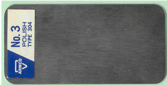
Photo 1 – Stainless Steel Type 304, No.3 Polish satisfactory for many industrial and commercial products requiring a good polished surface. Typical applications include vent hoods.
