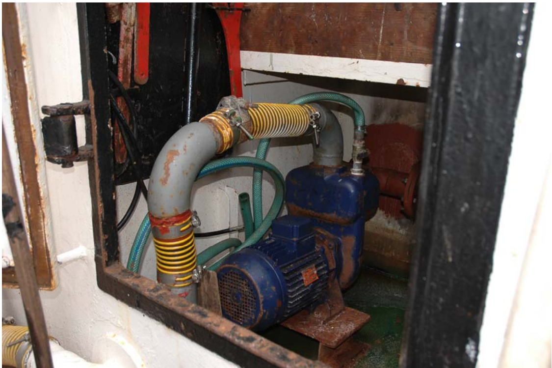
Plate 8: The water intake pipe for the CUFES on the “ RV Welwitchia ”
