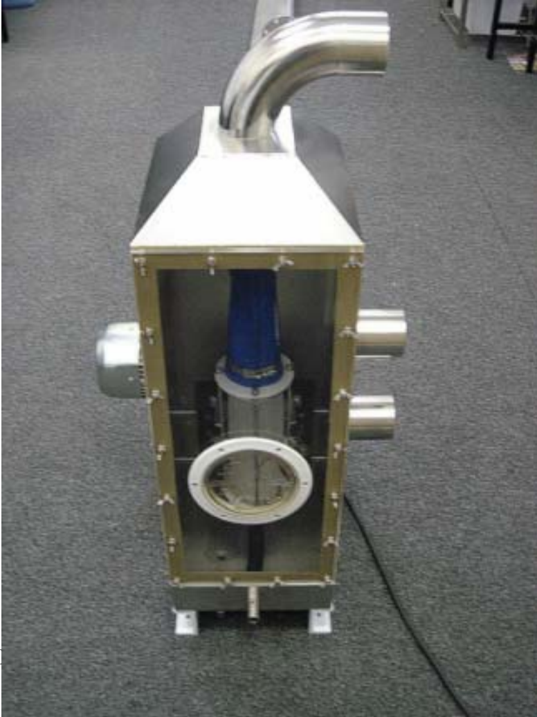
Plate 2: Stainless steel concentrator of the CUFES
