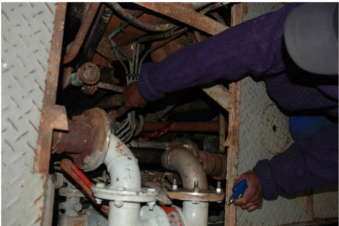
Plate 8: The water intake pipe for the CUFES on the “ RV Welwitchia ”
