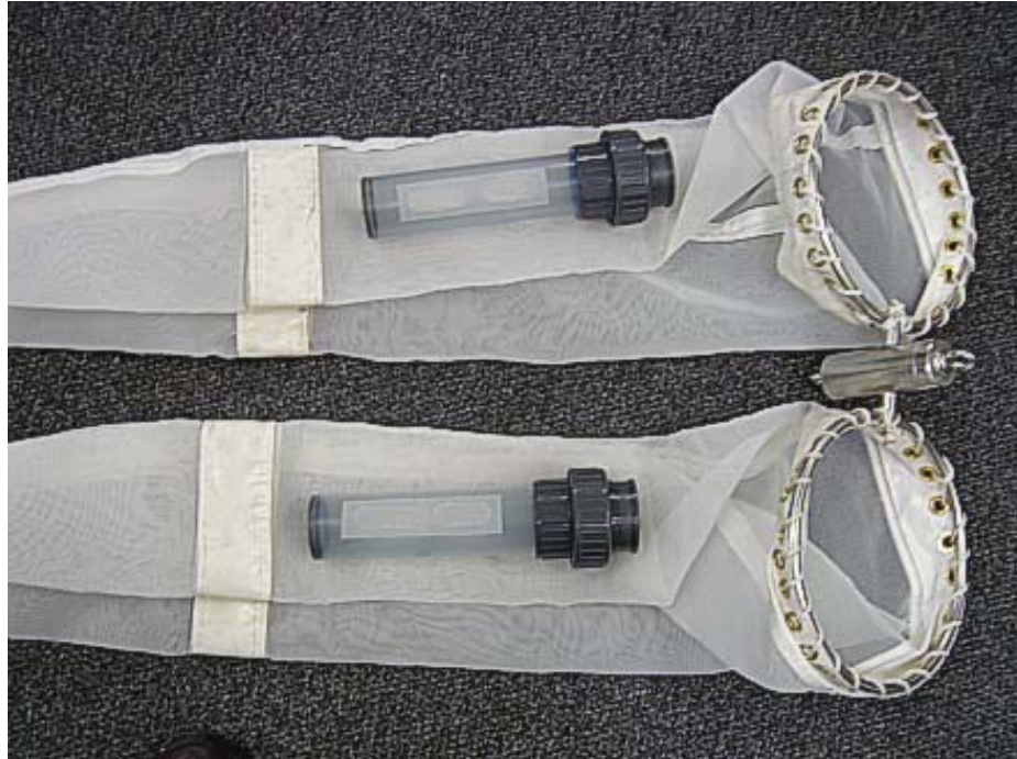
Plate 4: Double CalVET 25 cm diameter with stainless steel swivel / coupling between the rings.
