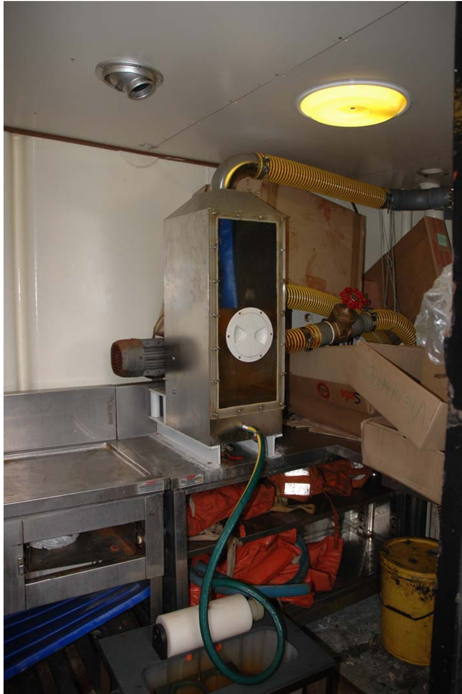
Plate 6: The concentration and sample collector in the laboratory on the “RV Welwitchia ”
