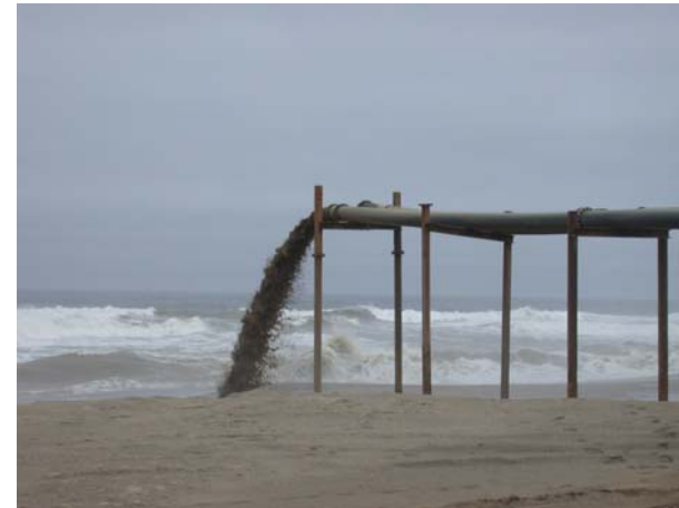
Plate 16. Discharge of high volumes of sediment into the sea from a land-based gravel processing facility in southern Namibia.
