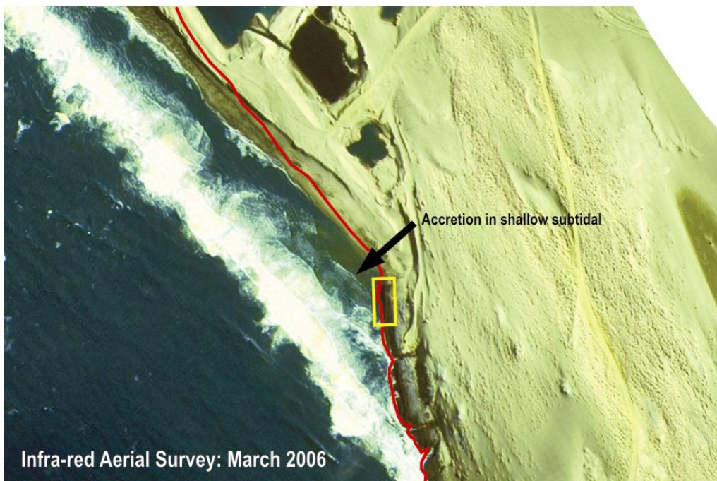
Figure 31. Aerial images of the southern portion of Pocket Beach 2, taken during the 2002 Airborne Lazer Survey (ALS), and 2006 Infra-red Aerial Survey of kelp beds, showing the beach accretion in the vicinity of the rocky intertidal sampling station (yellow rectangle). The red line represents the ALS low water mark, and is superimposed on the Infra-red image to illustrate the degree of beach accretion.
