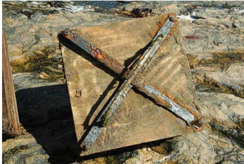
Plate 13: Corrosion of galvanised steel collector after a six-month period in the sea.
