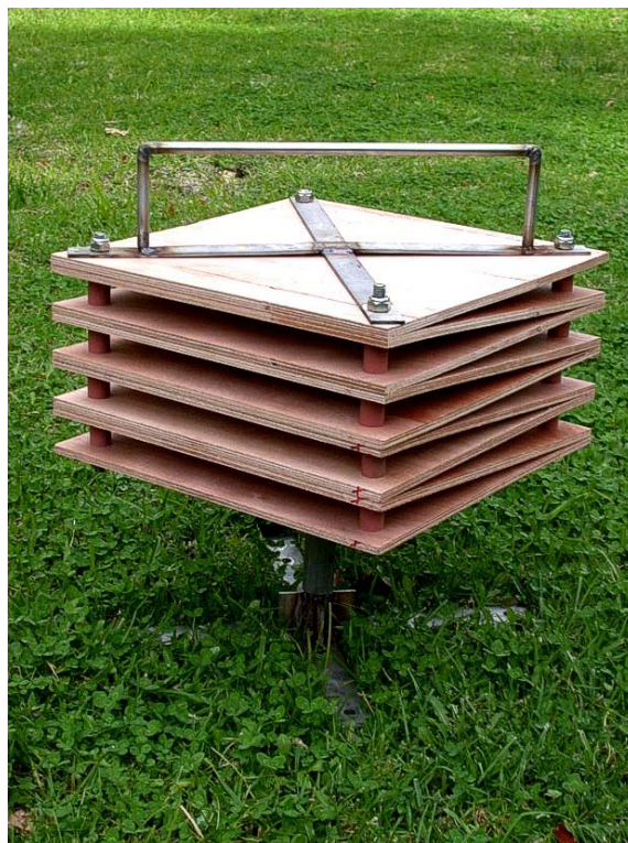
Plate 7. Booth crevice collector and base-plate made using stainless steel components.
