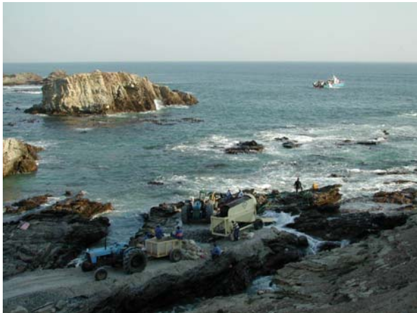
Plate 15. Typical shore-based contractor showing discard of fines across the intertidal and accumulation of tailings around the classifier. A vessel-based operation further offshore can also be seen.
