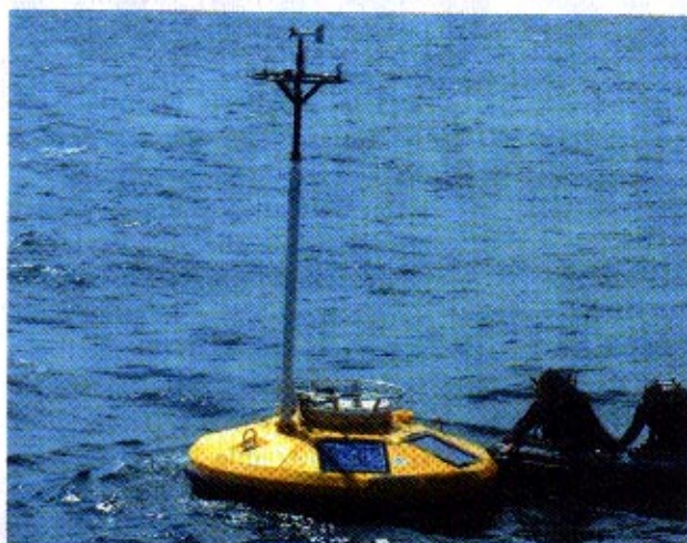
Moorings such as this Seawatch buoy will provide real-time data for an Early Warning System. (Credit: CSIR)
