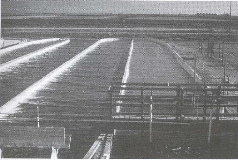
Figure 1–14 Microalgal production facility. Algal cultures are grown in successively larger volumes and finally cultivated for biomass harvest in long raceways stirred by paddle wheels (foreground). (Photograph courtesy J. Kranzfelder)
